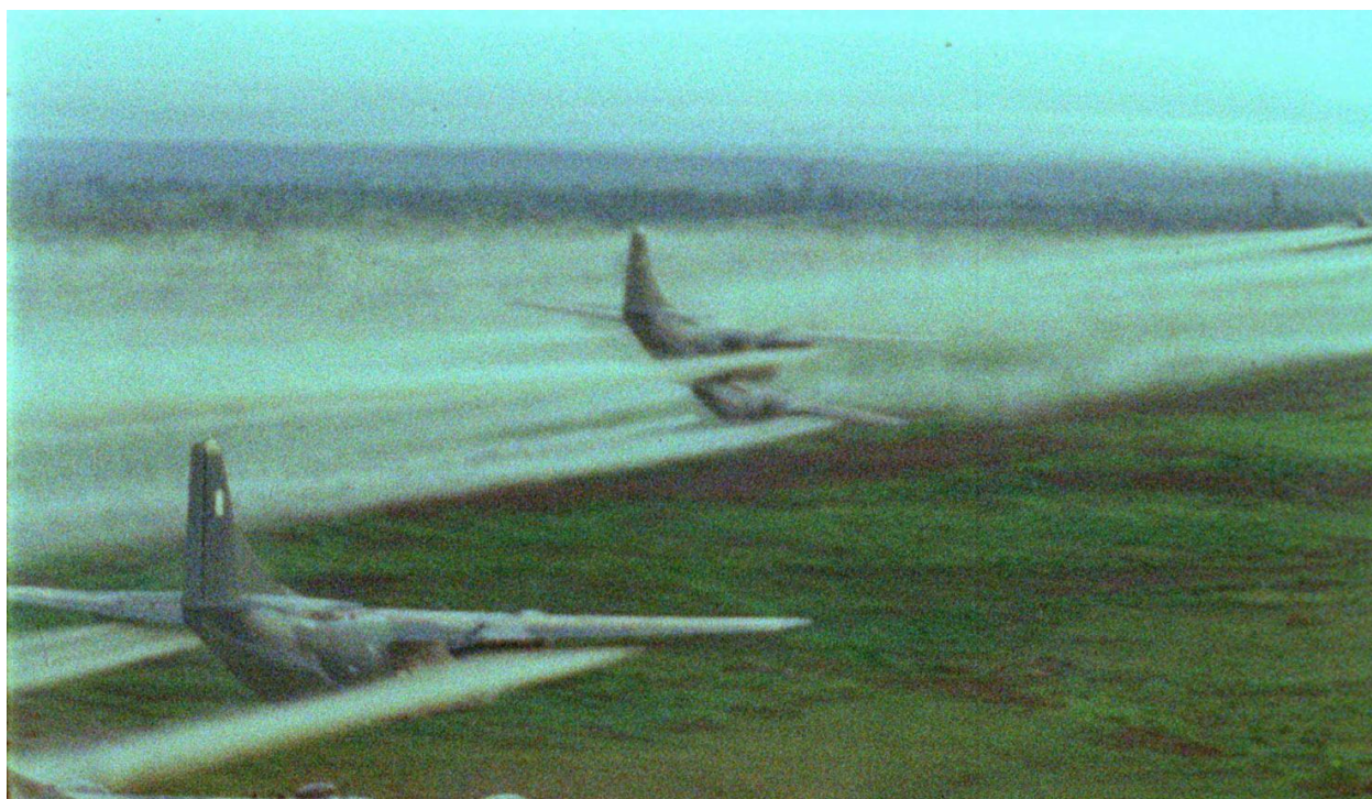
C-123 "Provider" aircraft spray Agent Orange, a 50/50 mixture of the herbicides 2,4,5-T and 2,4-D, over Vietnam during Operation Ranch Hand. Film still: US National Archives and Records Administration.
